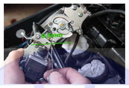
With the throttles still in the fully-closed position the TPS voltage should be 0.60V (+/- 0.02V). If the voltage is outside the range 0.58V - 0.62V adjustment is made by rotating the TPS, located on the left side of the throttle bodies.
