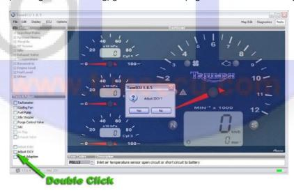
Confirm the "Adjust ISCV?" request. The Cyl 3 MP dial will change to a TPS Voltage indicator. TuneECU will send a command to move the throttles to the fully-closed position. If these checks are being performed because a new stepper motor has been fitted check the clearance between the idle speed control lever and the roller on the throttle cam. Clearance should be 0.5mm.
